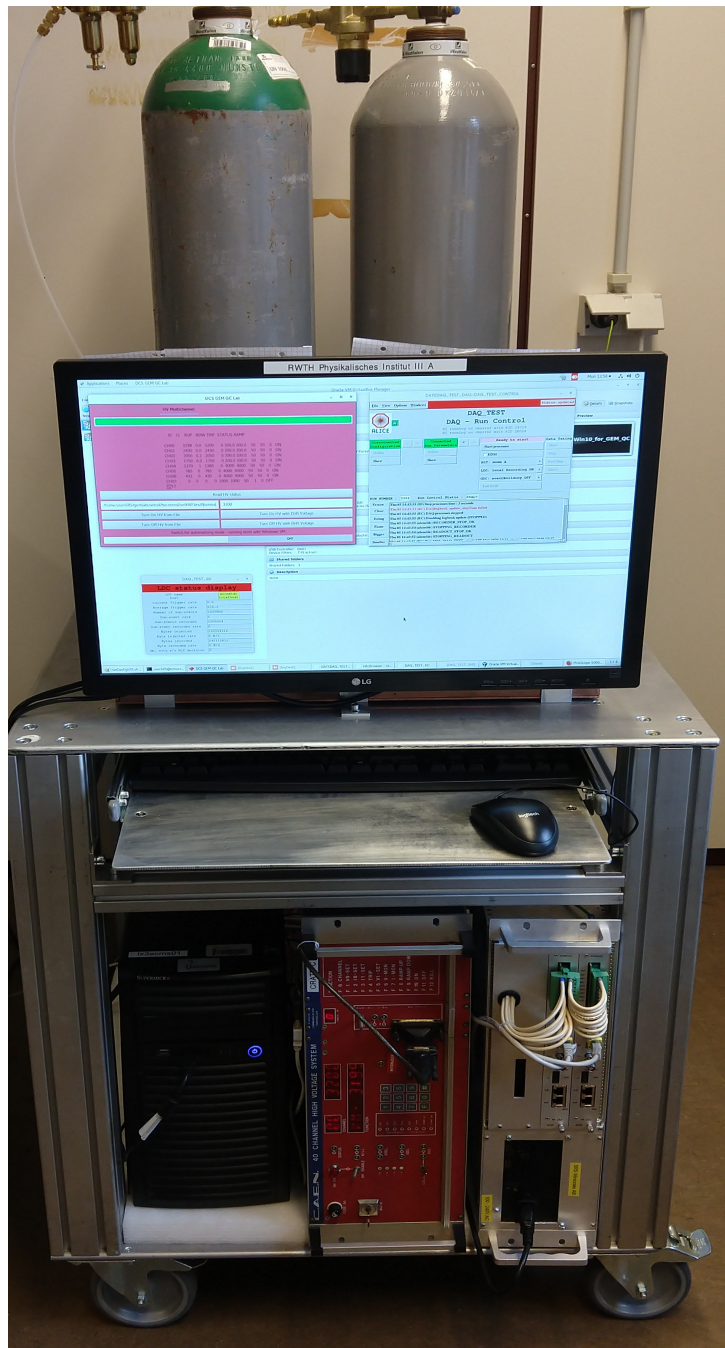
Figure (3.1) Experimental setup. On the bottom of the cart from left to right: the Desktop PC (black), CAEN HV system (red). On top of the cart can be seen the monitor attached to the copper enclosure with lines for the gas to the GEM chamber.
