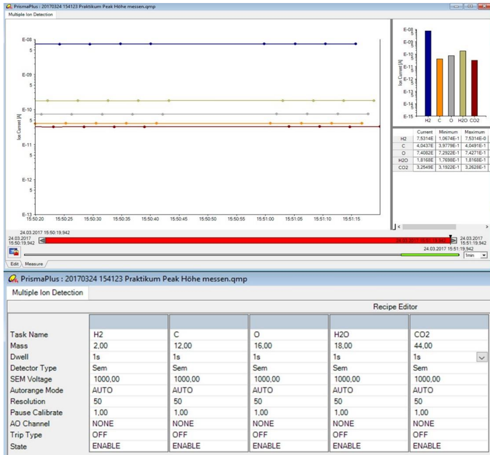
Fig. 3.2.3: QUADERA software: Template “Praktikum 5 Peak Höhen messen” and parameter edit window.
