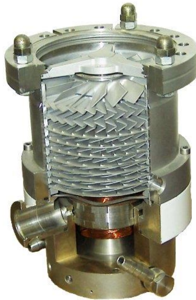
Fig. 2.1.2: View inside a turbomolecular pump [10].
