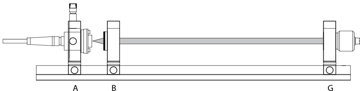
The objective of this first experiment is to set the semiconductor laser into operation. The laser module A is positioned on the optical rail as far to the left side as possible and clamped. The collimator B is put near the laser module and the photo detector G is mounted on the far right side of the optical rail. Never remove the photo diode G from the optical rail because it acts as a blocking element for the laser beam, so that it cannot leave the experimental area in an uncontrolled manner.
