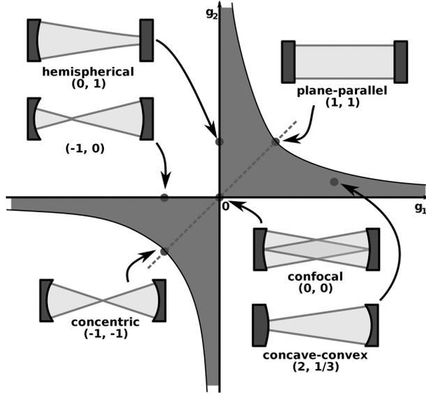
Figure 4: Stability diagram with different kind of resonators.
