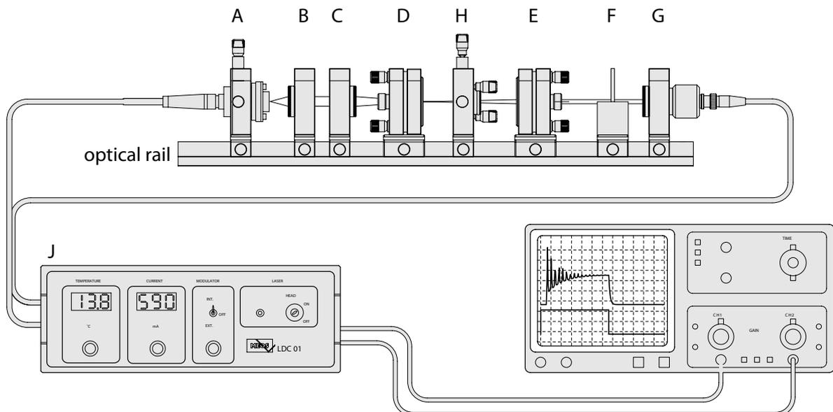
A The **diode laser module** consists of a XY adjustment unit in which the laser diode is mounted. A Peltier's cooling element for the control of the diode temperature and a thermistor for the measurement of the temperature are all located inside the laser diode. A warning lamp, which signals the presence of laser radiation, is fitted to the upper side of the module.
