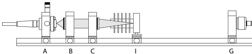
First move the photo detector (module G) back to the far right side of the optical rail. Remove module D and replace it with the power sensor (module I). **IMPORTANT:** Use the 1:1000 attenuator for this part of the experiment! This means the real, physical attenuator you have to mount on the photo-sensor, **NOT** the attenuation factor you can set in the electronic of the power meter (the latter one should ALWAYS be set to 1).
