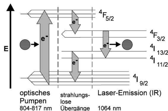
Figure 6: Important energy levels of the Nd<sup>3+</sup> ion for optical pumping with diode lasers and for the laser process.
