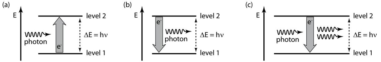
Figure 1: (a) Absorption of a photon. (b) Spontaneous emission of a photon. (c) Induced emission of a photon.
