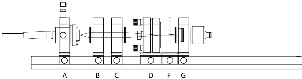
The initial level for emission with a wavelength of 1064 nm is the  ${}^4F_{3/2}$  level, which has a very long lifetime of about 230  $\mu\text{s}$  compared to normal optical transitions. If the Nd-YAG crystal is periodically pumped with the diode laser, then the variation of the spontaneous emission as a function of time can be displayed on an oscilloscope.
