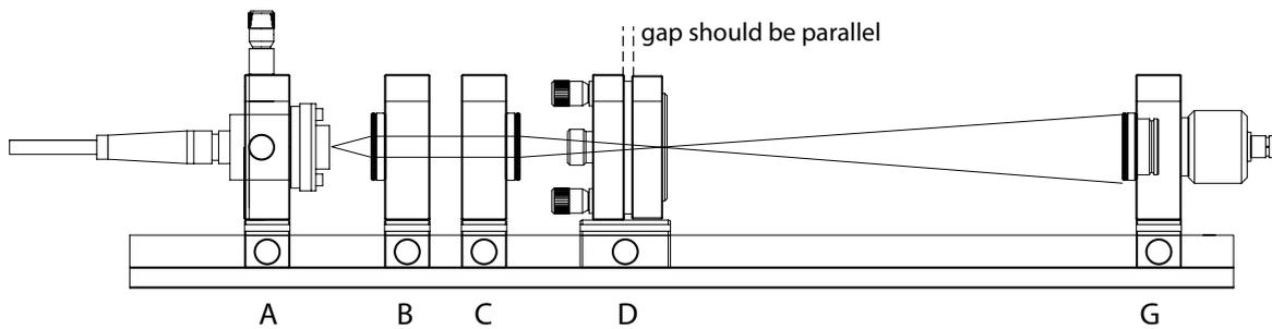
First check the modules D and E. Together these modules will create the resonator. The task of the corresponding adjustment holders is to align both mirrors in such a way that the optical axis of the resonator is perpendicular to the mirrors and parallel to the optical rail. In first order this is achieved when the gaps between the moveable and fixed plates of the adjustment holders are aligned parallel to each other.
