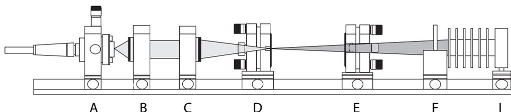
Check the modules D and E, which will form the resonator. The task of the corresponding adjustment holders is to align both mirrors in such a way that the optical axis of the resonator is perpendicular to the mirrors and parallel to the optical rail. In first order this is achieved when the gaps between the moveable and fixed plates of the adjustment holders are aligned parallel to each other.
