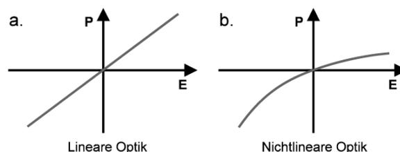
Figure 10: Polarization  $P$  of the dipoles in the presence of an electric field  $E$  in an optically linear (a) and a non-linear medium (b).
