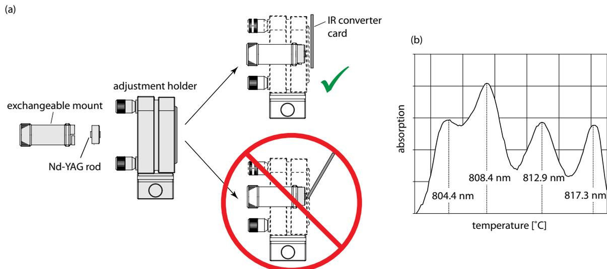
In the following experiment the dependence of the diode laser's wavelength on the diode temperature is determined. For this the well-known absorption lines of the Nd-YAG crystal are used. There are four absorption transitions which can (in principal) be pumped with the laser diode used in this experiment. The maxima of the absorption spectrum are located at: 804.4 nm, 808.4 nm, 812.9 nm, and 817.3 nm.
