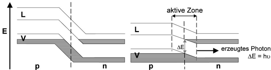
Figure 7: The pn junction of a semiconductor diode with the conduction band L and valence band V. Left without applied voltage, right with applied forward voltage. The active region contains both electrons and holes which generate photons by recombination.
