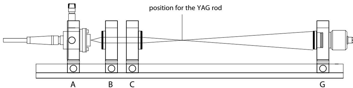
Next the focusing unit is positioned on the optical rail. This unit contains a biconvex lens with a focal length of 60 mm. Later on it is used for focusing the diode laser beam into the Nd-YAG rod. Set up the focusing module at a distance of about 50 – 100 mm from the collimator.
