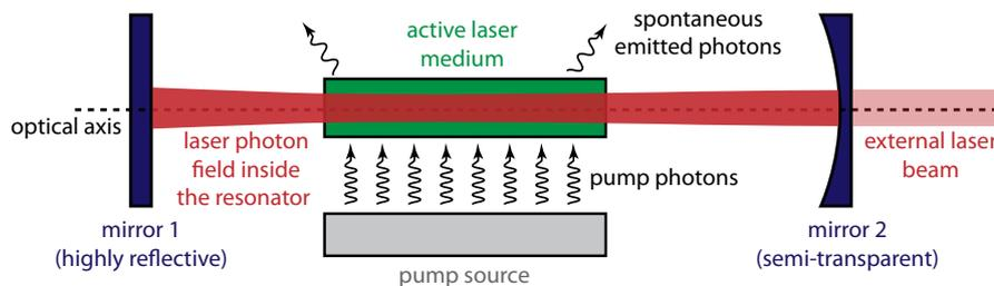
Figure 3: Optically pumped active medium inside an optical resonator.
