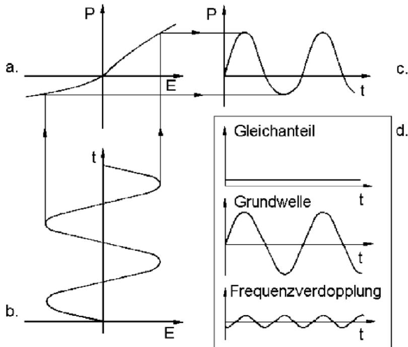
Figure 11: An electron with a non-linear polarization characteristic (a) is exposed to a sinusoidal external field strength (b). Hence, the time dependency of the polarization and therefore the vibration of the electron is non-harmonic (c). The Fourier decomposition of the non-harmonic oscillation yields a DC, a linear and a frequency-doubled contribution (d).
