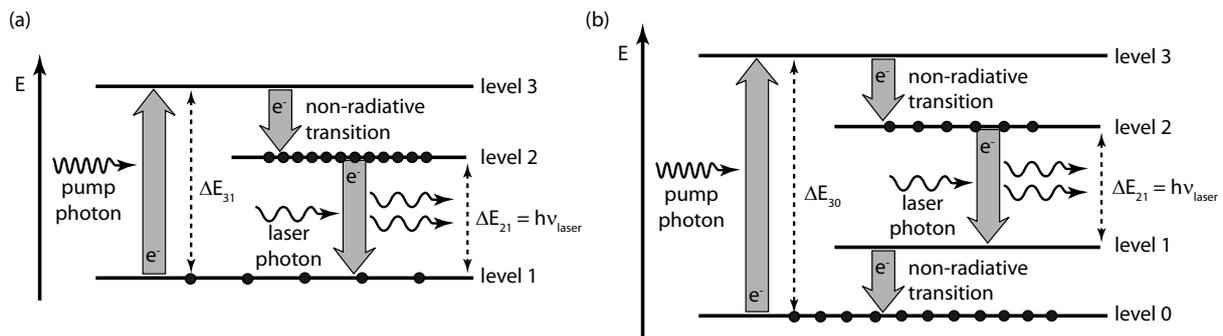
Figure 2: (a) Schematic diagram of a (a) three-level laser system and (b) four-level laser system.
