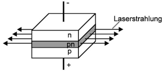
Figure 8: Schematic diagram of an injection laser.
