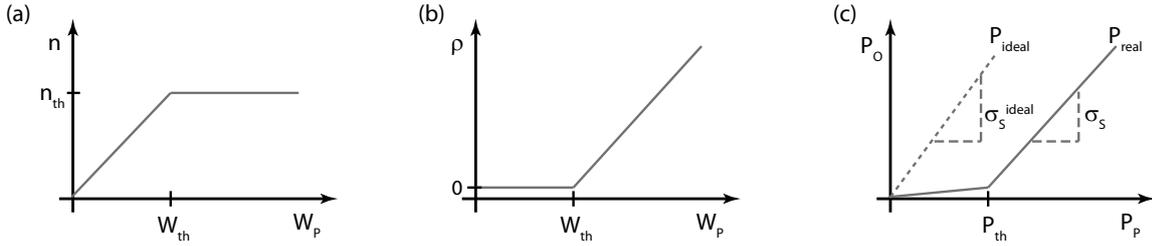
Figure 5: (a) Inversion  $n$  as a function of pump rate  $W_p$ . (b) Photon density  $\rho$  as a function of pump rate  $W_p$ . (c) Laser output power  $P_o$  as a function of pump power  $P_p$ .
