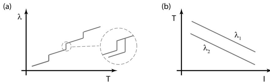
Figure 9: (a) Emitted wavelength  $\lambda$  of a diode laser as a function of crystal temperature  $T$ . Inset shows the hysteresis effect. (b) Curve of constant wavelengths as a function of temperature  $T$  and the injection current  $I$  of a semiconductor laser.
