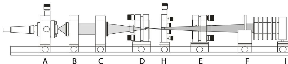
If the previous experiments were conducted with the R100-2 mirror, swap it with the SHG100 mirror. Keep in mind that the intensity of the fundamental wave should be as high as possible for an efficient frequency doubling.
