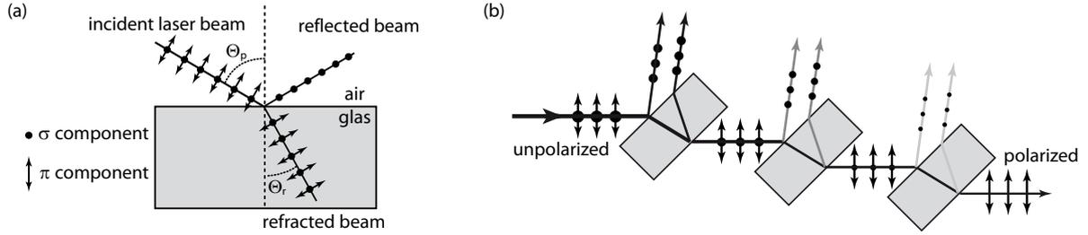
Figure 5: (a) Illustration of the polarization of a light beam which hits the surface of a glass slide at the Brewster angle. (b) Polarization of a light beam by subsequent transmission through a glass slide.
