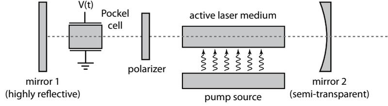
Figure 4: Schematic of a laser system with a Pockels cell as an optical switch for pulse generation.
