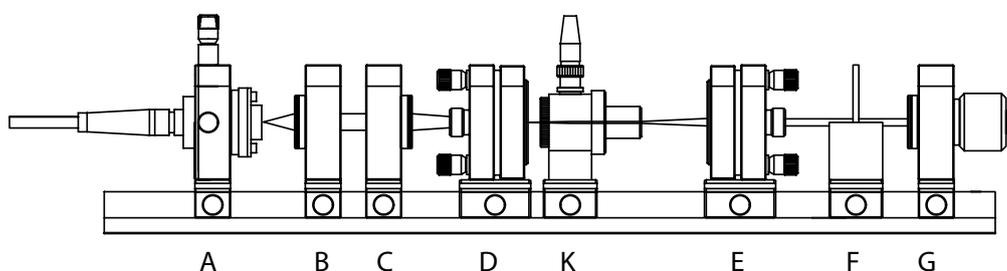
In the next step, put the Brewster window on the Pockels cell, but do not tighten the screw yet. Then connect the Pockels cell to its driver and the driver to the function generator. Set the frequency of the function generator to 1 kHz.
