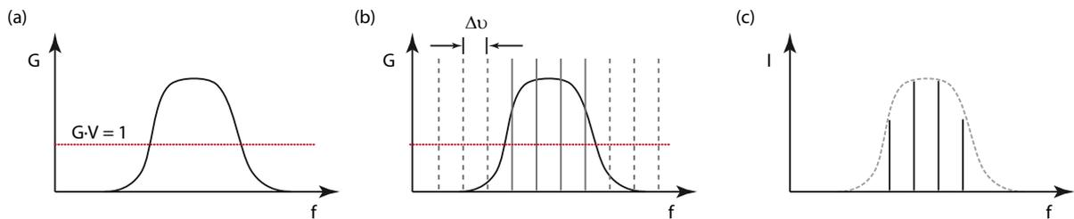
Figure 6: (a) Schematic laser bandwidth spectrum with the amplification threshold  $G \cdot V = 1$ . (b) as in (a) but with the longitudinal modes of the optical resonator. (c) Resulting laser output spectrum.
