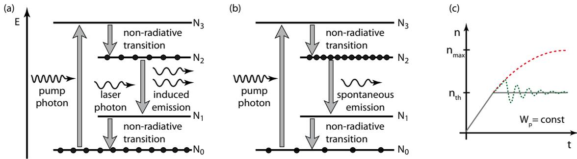
Figure 1: Schematic diagram of a four-level laser system with (a) and without (b) optical resonator. (c) Population inversion with an optical resonator under ideal conditions (gray solid line), with an optical resonator with transient effects (green dotted line) and without an optical resonator (red dashed line) as a function of time at a constant pumping power.
