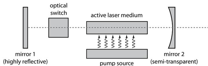
Figure 3: Schematic of a laser system with an optical switch for pulse generation.
